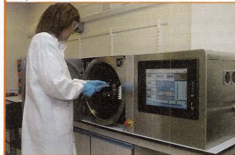
Figure 1: Loading a plasma processing system with polymer components.
